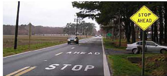
Figure 24: Advanced warning signage on a rural road; image source: FHWA
