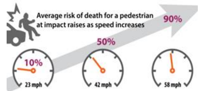
Figure 58: AAA Foundation for Traffic Safety, Impact Speed and the Pedestrian's Risk of Severe Injury or Death , September 2011.
