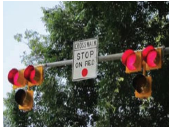
Figure 46: Pedestrian Hybrid Beacon (PHB); image source: FHWA
