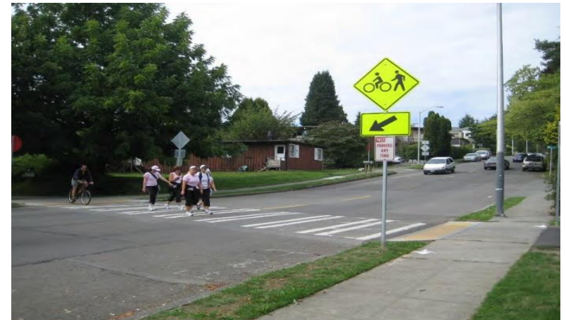
Figure 44: Signage and markings at a designated crosswalk; image source: City of Fresno
