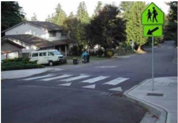
Figure 45: Curb extension along a crosswalk; image source: FHWA
