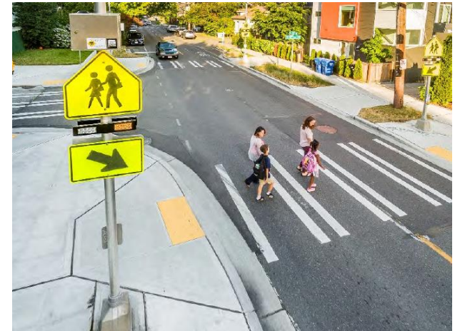
Figure 47: Rectangular Rapid Flashing Beacon (RRFB) along a crosswalk; image source: City of Fresno
