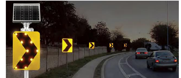
Figure 37: Flashing beacons on chevron signs along a curve; image source: Marin County
