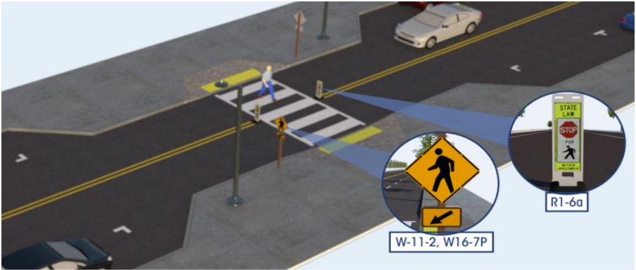
Figure 42: A variety of crosswalk visibility enhancements at a pedestrian crossing; image source: FHWA
