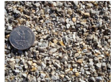
Figure 19: Close up of aggregate used in HFST; image source: FHWA
