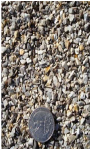
Figure 33: Close up of aggregate used in HFST; image source: FHWA
