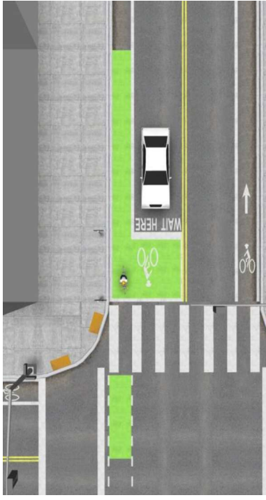
Figure 50: A bike box at an intersection; image source: National Association of City Transportation Officials; nacto.org
