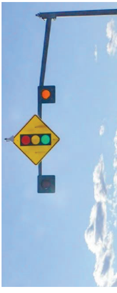
Figure 18: A flashing beacon; image source: Marin County
