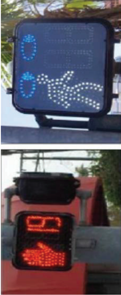
Figure 41: Two styles of pedestrian countdown signal heads; image source: FHWA
