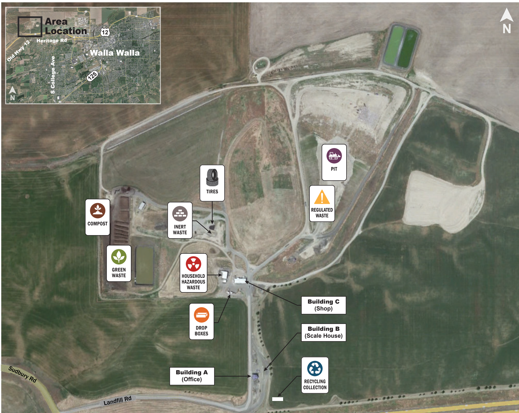
Figure 5-1. Sudbury Road Landfill: Existing Site Layout
