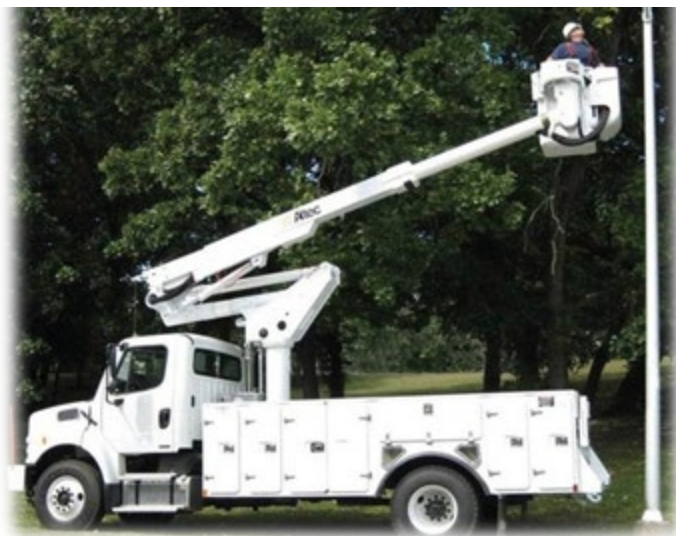
Aerial Cable Placement (Bucket Truck)
