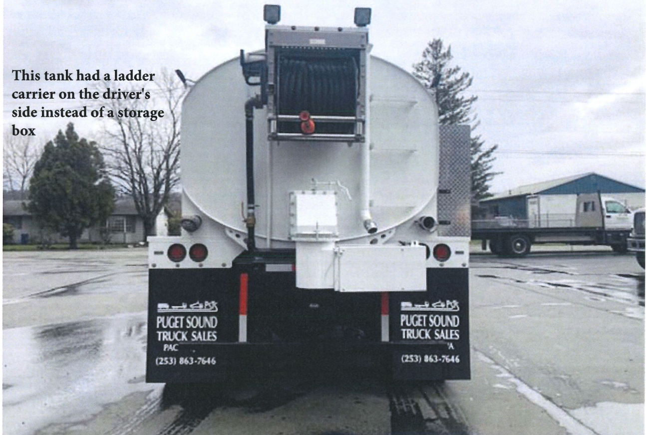
View of narrowed tank design allowing driver's side storage box and passenger side porta tank carrier.
