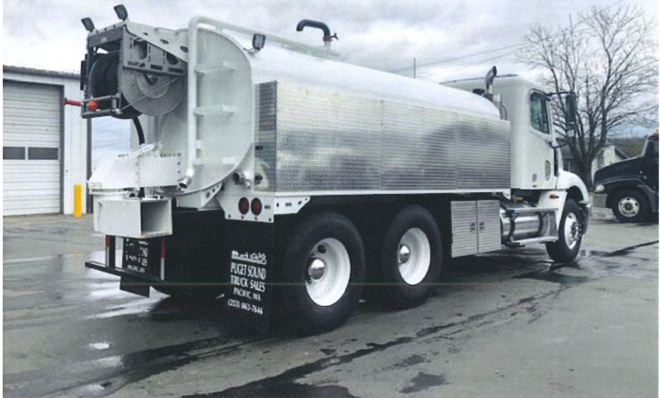
Prior unit built- similar tank design. Showing the porta tank carrier arrangement
