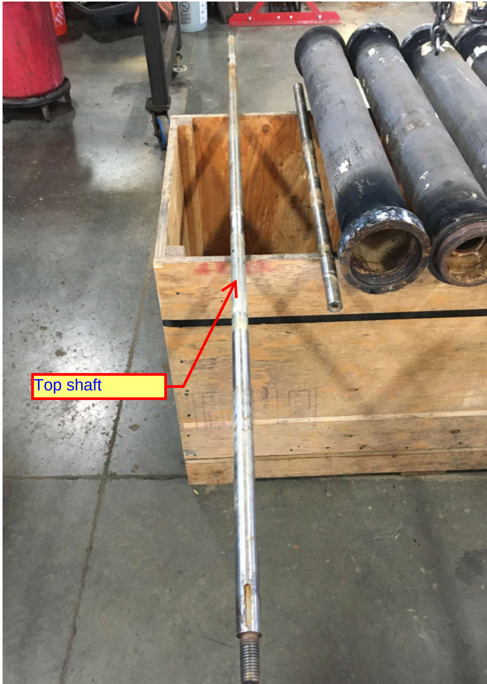
Top shaft, key way and step down for motor coupling
